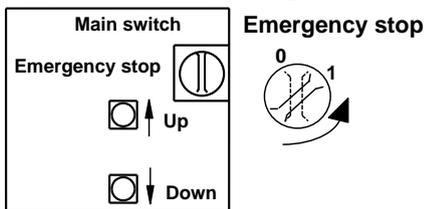
An easily and quickly accessible emergency stop device needs to be available at each control-section. Where required, additional devices for an emergency stop need to be installed, for example in the vicinity of unprotected cable winches.
