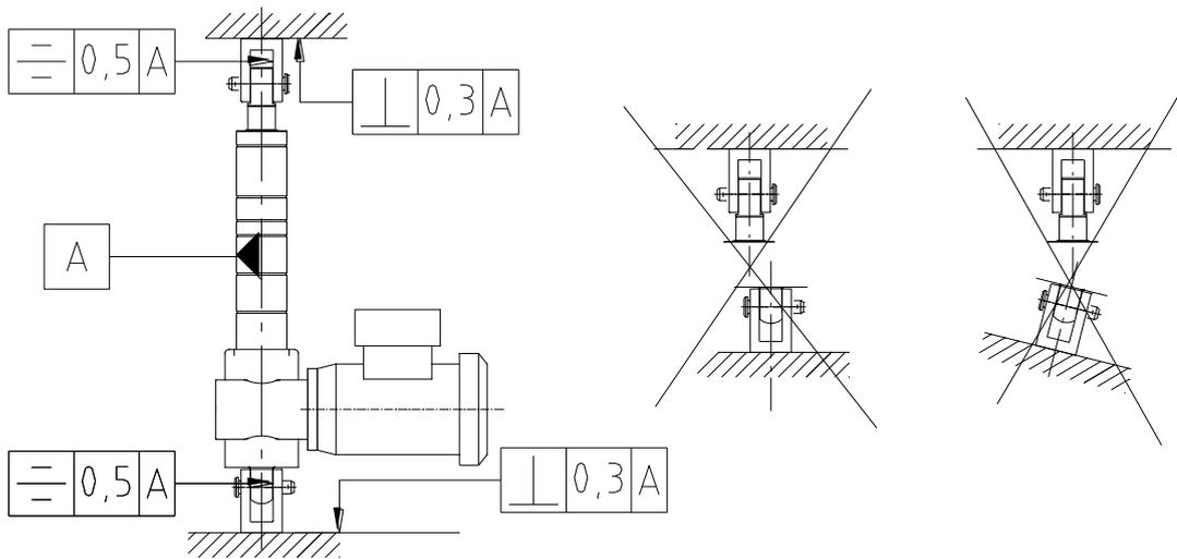
**4.1 Mechanical fastening of the console (only for sizes 20.1 and 30.1)**
