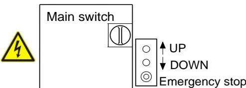
**In any case, a quickly accessible emergency off button (switch) needs to be implemented (integrated in Pfaff-silberblau controls).**
